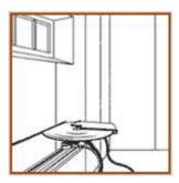
• Cut the window opening with a concrete saw. Make the opening 1/2" larger in width and height than the window unit.
