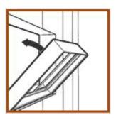
• Install the window from the interior. Make if flush with the inside of the wall. Install with: Shims, Concrete Anchor Bolts, Neutral Cure Silicone Sealant
